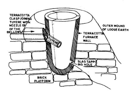
Fig. 1 Assembled copper smelting furnace from Avaram
